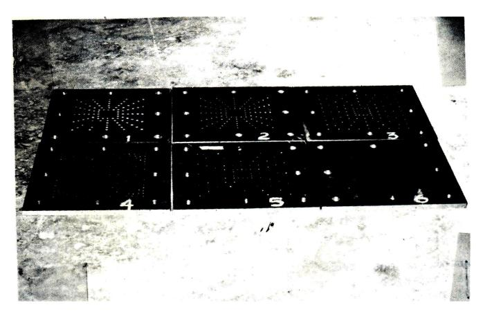
Fig. 3. Samples of Die base plates with various vent distributions
