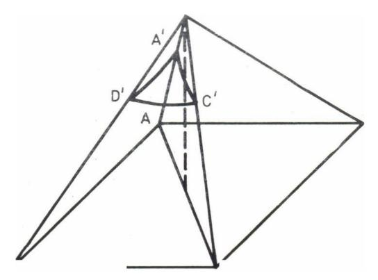
Fig. 1. Solid angle substended by square blank ABCD at charge center O
