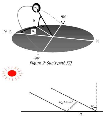
Figure 3. Angle of incidence u of the solar radiation [6]
