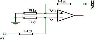
Figure 11 Comparator circuit
