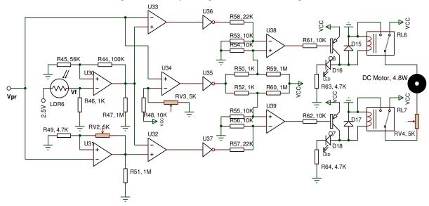
*Figure 7: Movement controller circuit diagram*
