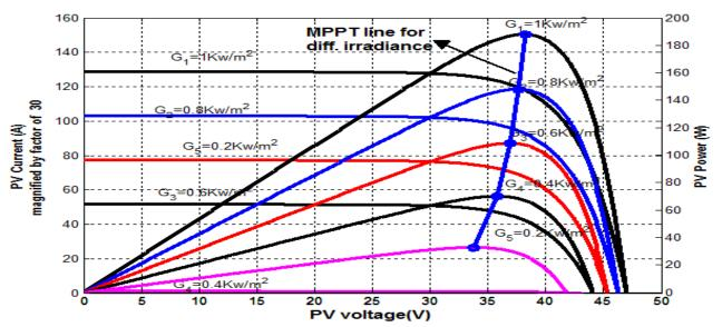
Figure 1: MPPT at different irradiance for I-V & P-V of PV panel at constant temp. of 25°C
