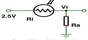
*Figure 10 Voltage divider network* Consider the circuit in figure 10.
