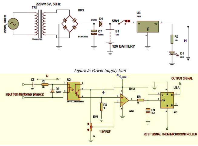
Figure 6: Blown Fuse Detector Circuit.
