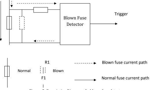
Figure 2: Descriptive Diagram of a blown fuse detector.
