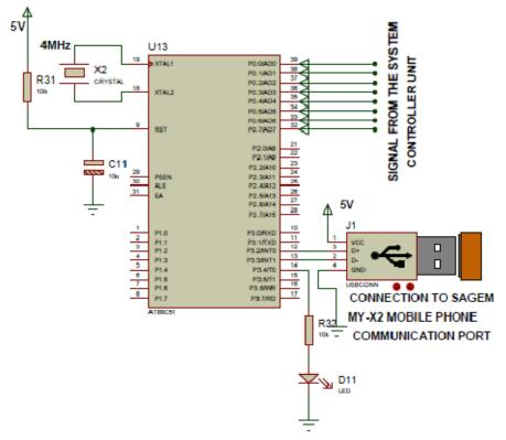
Figure 8: SMS controller Unit.
