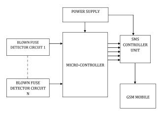
Figure 4: Block Diagram of GSM based transformer phase monitoring system
