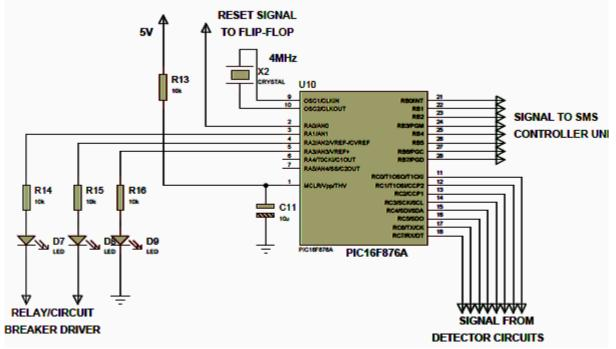
Figure 7: Systems Controller Unit.
