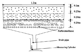
Figure 1: Schematic diagram of sand drying bed.
