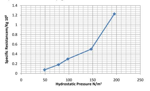
*Figure 4, Plot of specific resistance against Hydrostatic pressure.*
