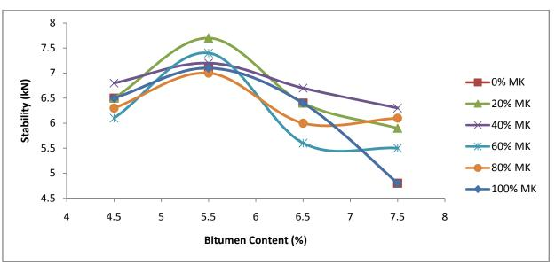
Figure 3: Combined Graph of Stability Vs Binder content
