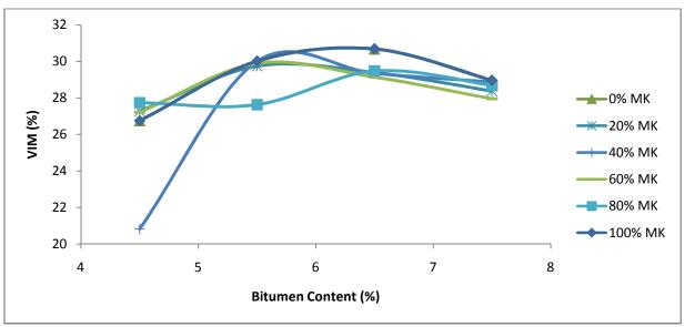
Figure 6: Combined Graph of VIM Vs Binder content
