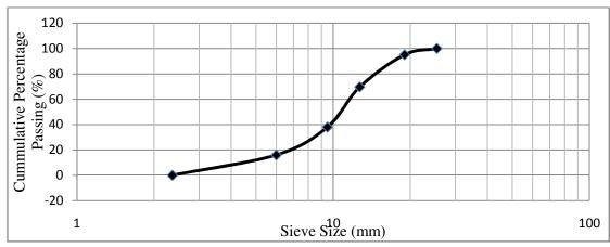
Figure 1: Particle Size Distribution Curve for Coarse Aggregate
