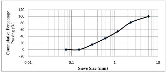
Figure 2: Particle Size Distribution Curve for Fine Aggregate
