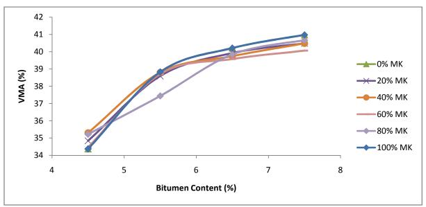
Figure 7: Combined Graph of VMA Vs Binder content.
