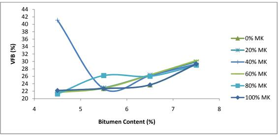
Figure 8: Combined Graph of VFB Vs Binder content
