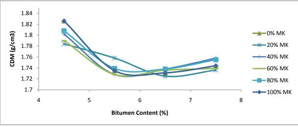
Figure 5: Combined Graph of CDM Vs Binder content.
