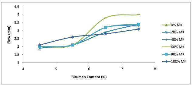
Figure 4: Combined Graph of Flow Vs Binder content
