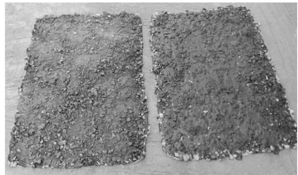
Figure 9: Final product of locally produced cold patch road mat
