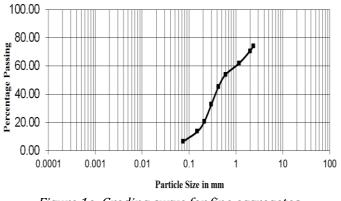
Figure 1a: Grading curve for fine aggregates
