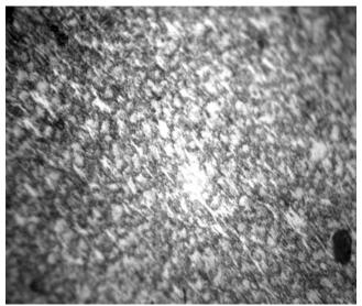
Plate 2: Photomicrograph of B730 X400 i.e. Sample intercritically annealed at 730°C for 30 minutes. The structure reveals large proportion of ferrite (light) matrix and martensite (gray) with little retained austenite (dark).
