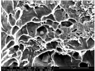
*Plate 7: Fractograph of sample B750 showing ridge – like features with more of cleavage surfaces.*
