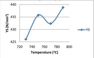
Fig. 4: Yield Strength (N/mm<sup>2</sup>) against Temperature (°C)
