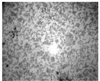
Plate 1: Photomicrograph of A X400 i.e. phase structure produced by normalizing at 850°C for one hour. The structure reveals ferrite (light phase) and pearlite (alternate layers of ferrite - light and cementite – dark).
