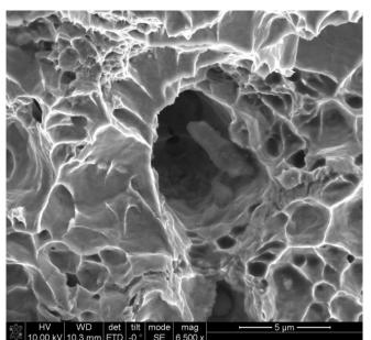
*Plate6: Fractograph of sample A showing a mixture of fibrous and cleavage surfaces.*
