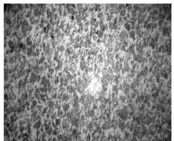
Plate 3: Photomicrograph of B750 X400 i.e. Sample intercritically annealed at 750°C for 30 minutes. The structure reveals large proportion of ferrite (light) matrix and increased number of martensite (gray) with little retained austenite (dark).
