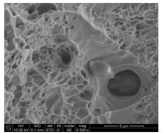
*Plate 9: Fractograph of B770 Structure reveals dimple fibrous fractured surface.*
