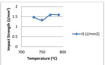
*Fig. 2: Impact Strength (toughness) (J/mm<sup>2</sup>) Versus Temperature (°C)*
