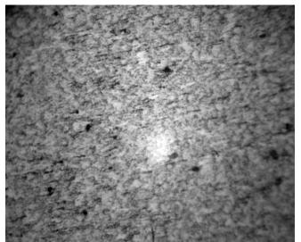
Plate 5: Photomicrograph of B790 X400 i.e. Sample intercritically annealed at 790°C for 30 minutes. The structure reveals fine distribution of ferrite (light) matrix and martensite (gray) with little retained austenite (dark).
