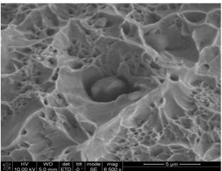
*Plate 8: Fractograph of B790: Structure reveals dimple fibrous fractured surface.*
