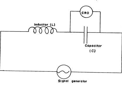
FIG.1. Experimental arrangement for the measurement of dielectric constants
