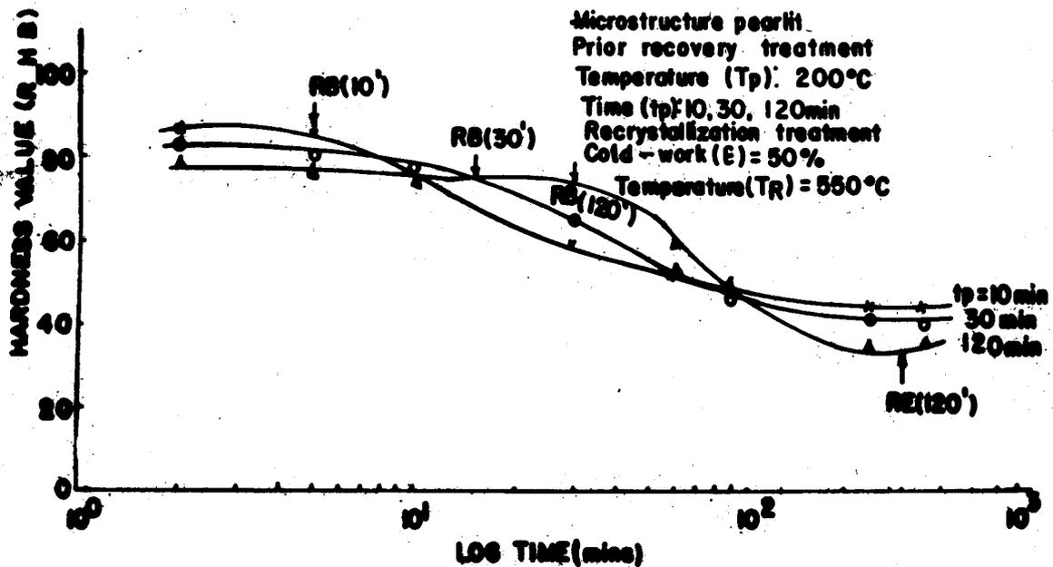
Figure 3. variation of hardness with time during recrystallization annealing of a pearlitic microstructure after previous recovery heat-treatment for various times,  $t_p$ . (% Deformation = 50;  $t_p$  = 10min, 30min, 120min.)
