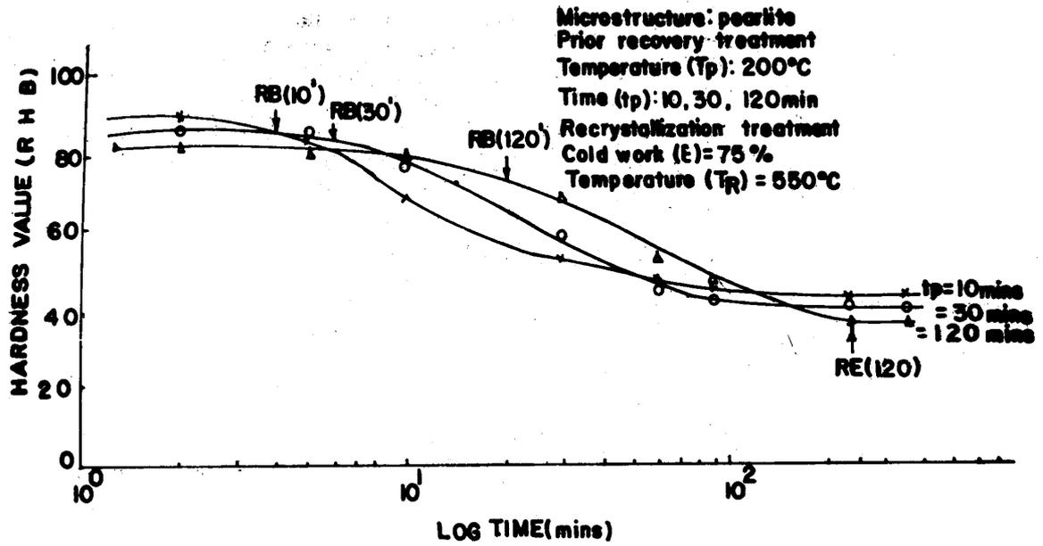
Figure 4. Variation of hardness with time during recrystallization annealing of a pearlitic microstructure after previous recovery heat-treatment for various times,  $t_p$ . (% Deformation = 75;  $t_p$  = 10min, 30min, 120min.)
