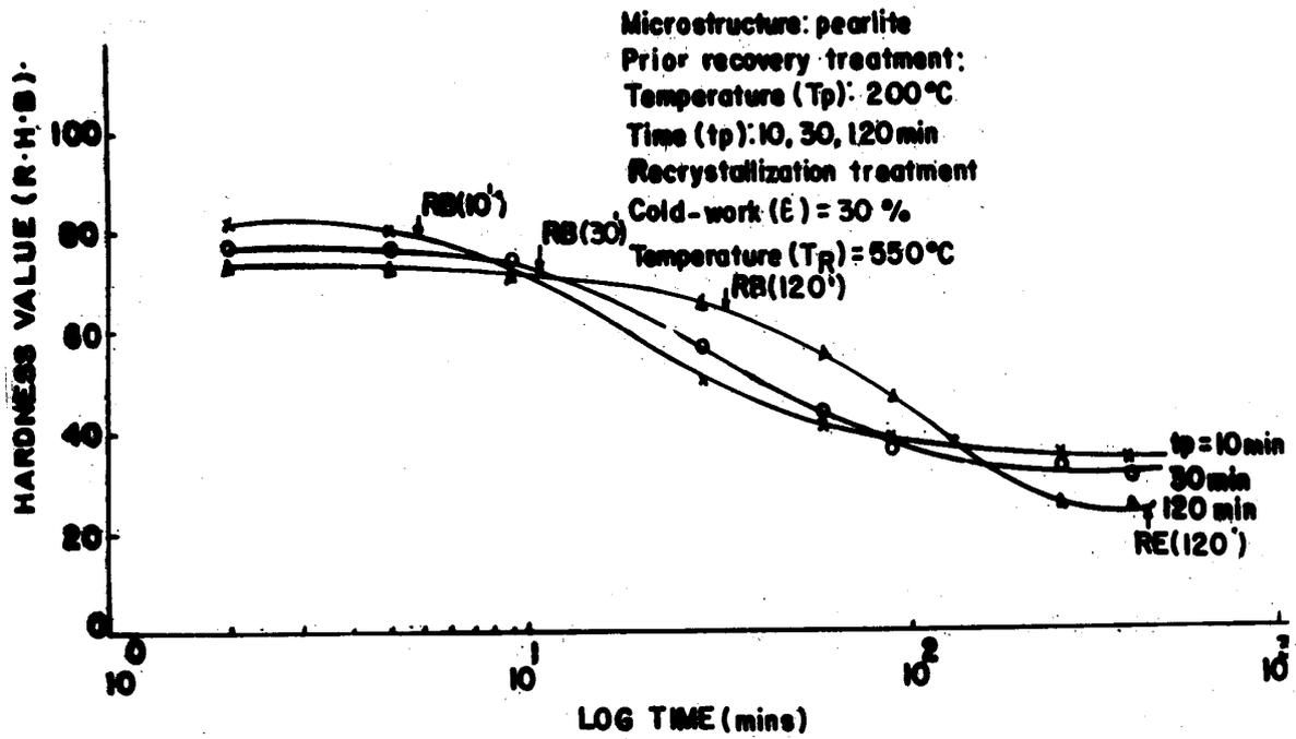
Figure 2. Variation of hardness with time during recrystallization annealing of a pearlitic microstructure after previous recovery heat-treatment for various times,  $t_p$ . (% Deformation = 30;  $t_p$  = 10min, 30min, 120min.)
