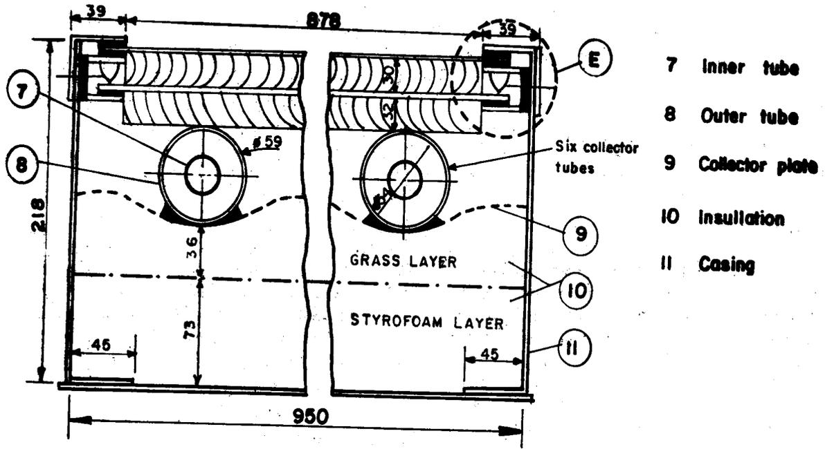
END SECTION Showing rubber seals, collector tubes & plate and insulation layers.
