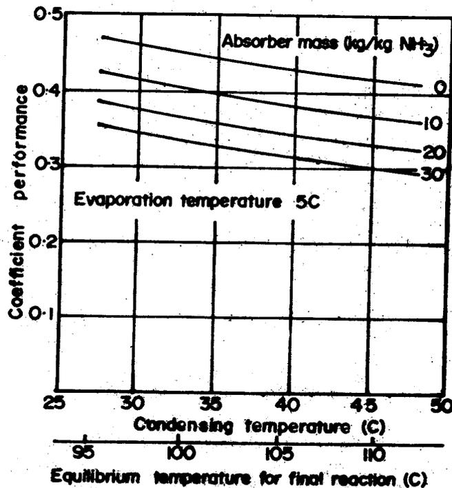
Figure 5: Coefficient of performance of the calcium chloride/ammonia cycle with different absorber mass ratio (mass of steel in absorber tubes and collector plates per unit mass of desorbable ammonia. For a practical design the mass ratio is about 10-20 [30])
