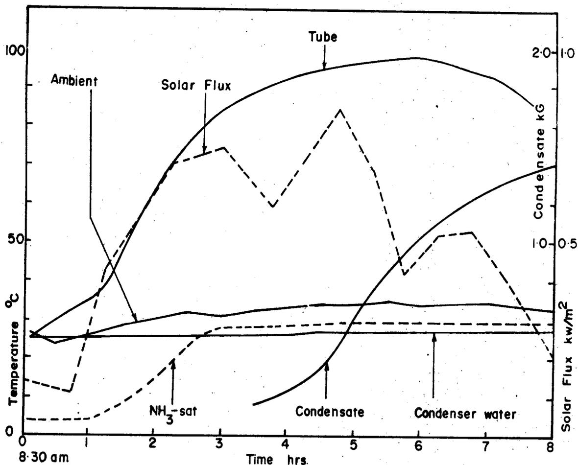
Figure 3. Temperature Profiles During Generation in Sunny Dry Season, Run #31.
