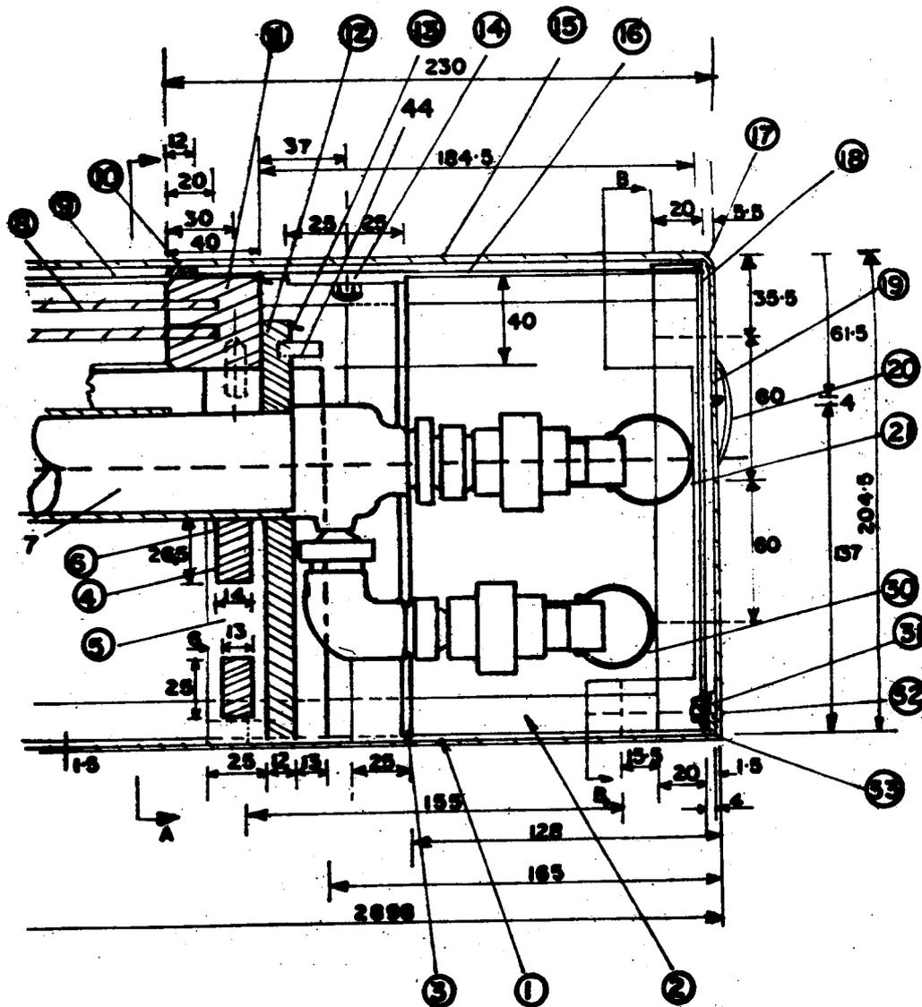
Figure 6: Longitudinal Cross-Section of new Collector (Scale x1/2mm)
