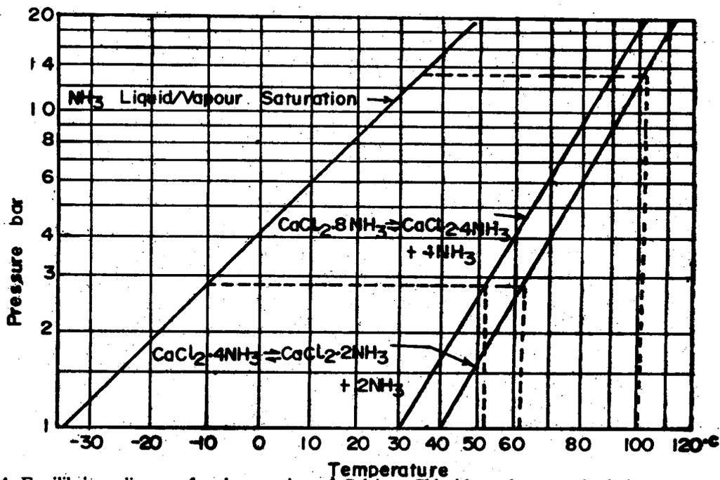
Figure 4: Equilibrium diagram for the reaction of Calcium-Chloride and Ammonia (10).
