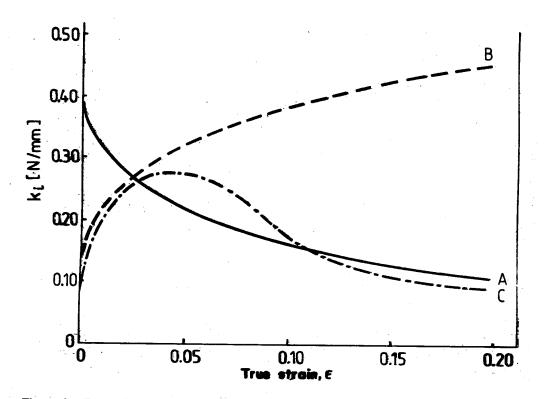
Figure 2a: Dependence of Hall – Petch Slope on Strain. A, B, C refer to austenitic steel of low, high and medium SFE respectively. (Dollar and Gorczyka, 1985)
