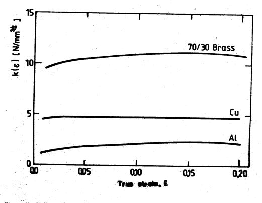
Figure 2b: Hall - Petch Slope versus True Strain (Hansen, 1985)
