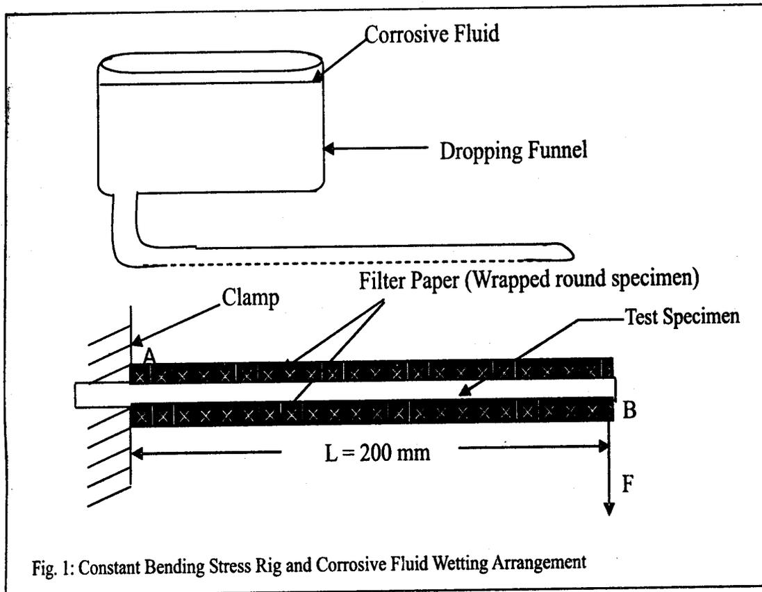
Fig. 1: Constant Bending Stress Rig and Corrosive Fluid Wetting Arrangement
