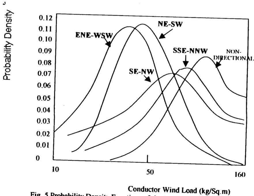
Fig. 5 Probability Density Functions of the Extreme Wind Loads for Typical line Orientations
