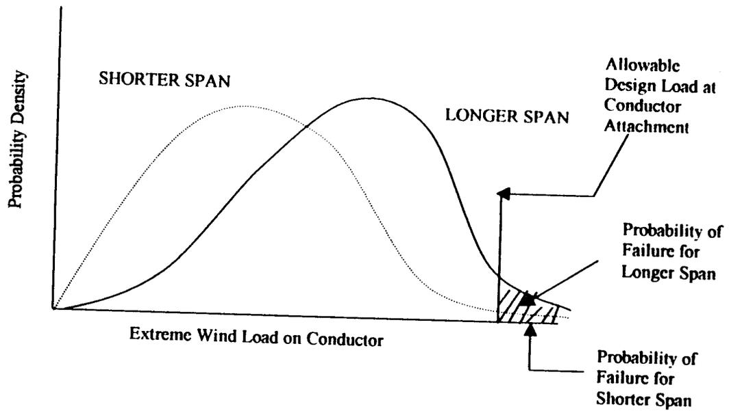
Fig. 6 Concept of the Probability of Tower Failure under Transverse Wind Loads
