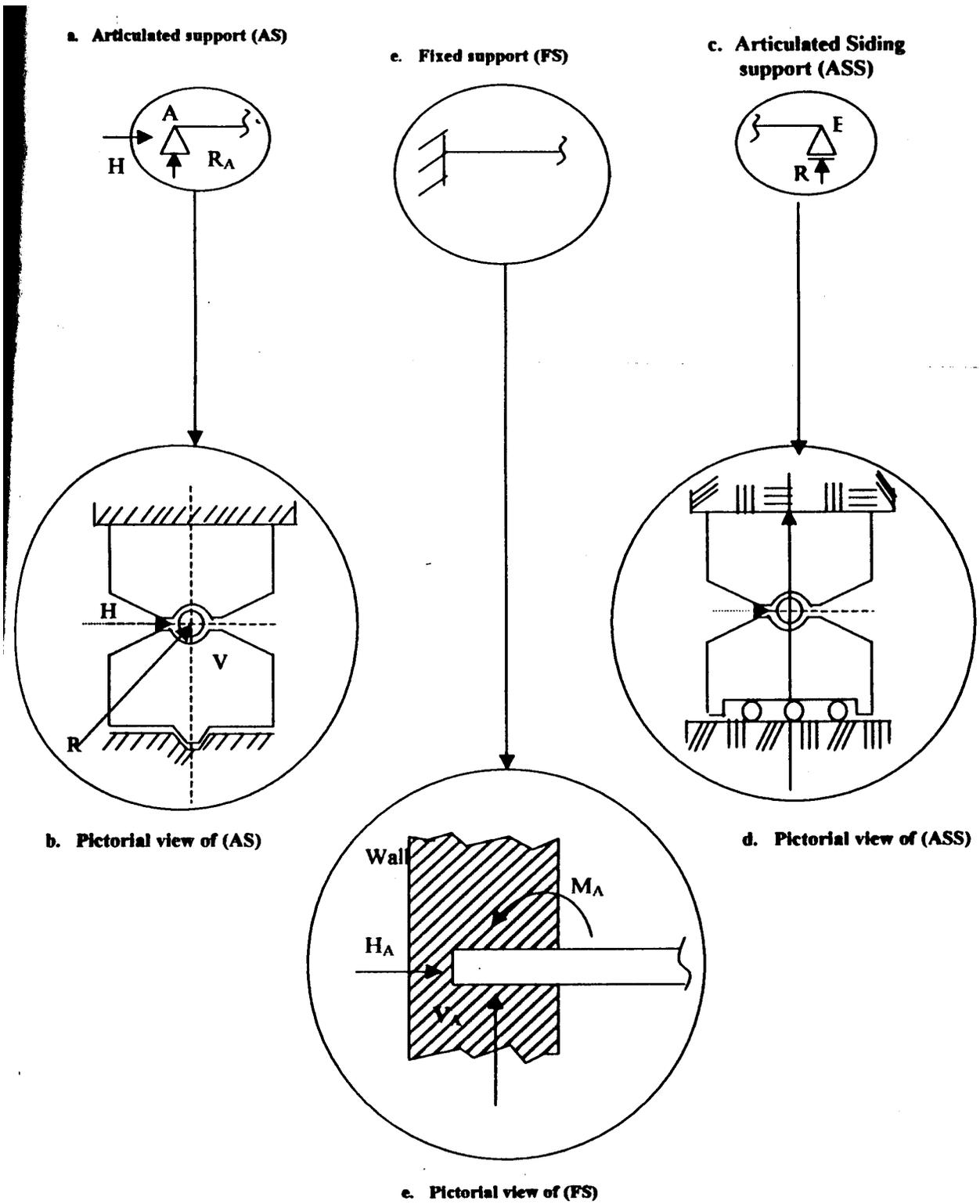
Fig.2. non –deformable rigid supports
