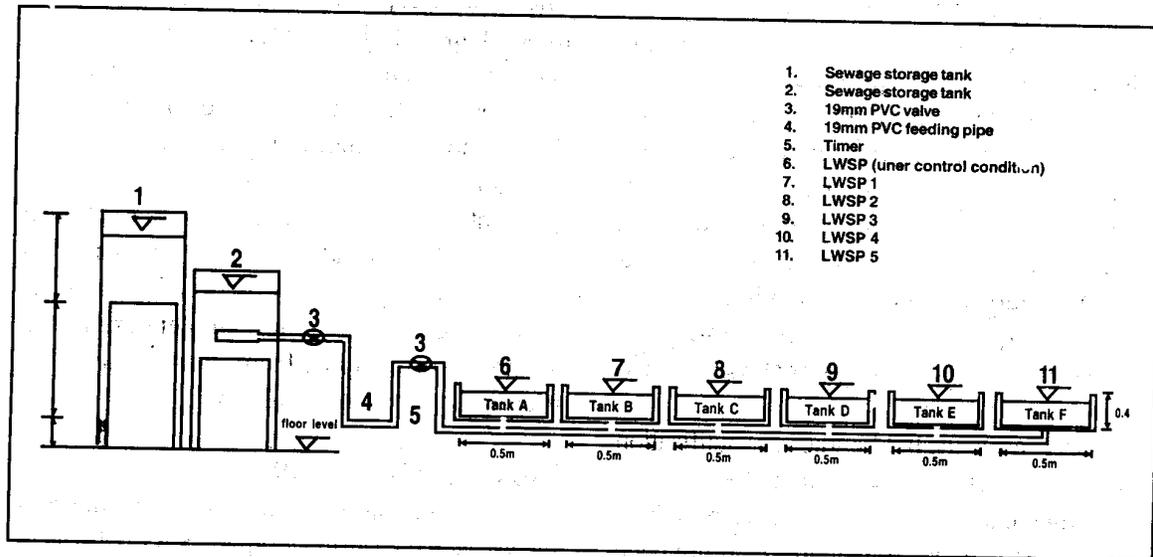
Fig. 1: vertical profile of LWSP for the study of thermal stratification
