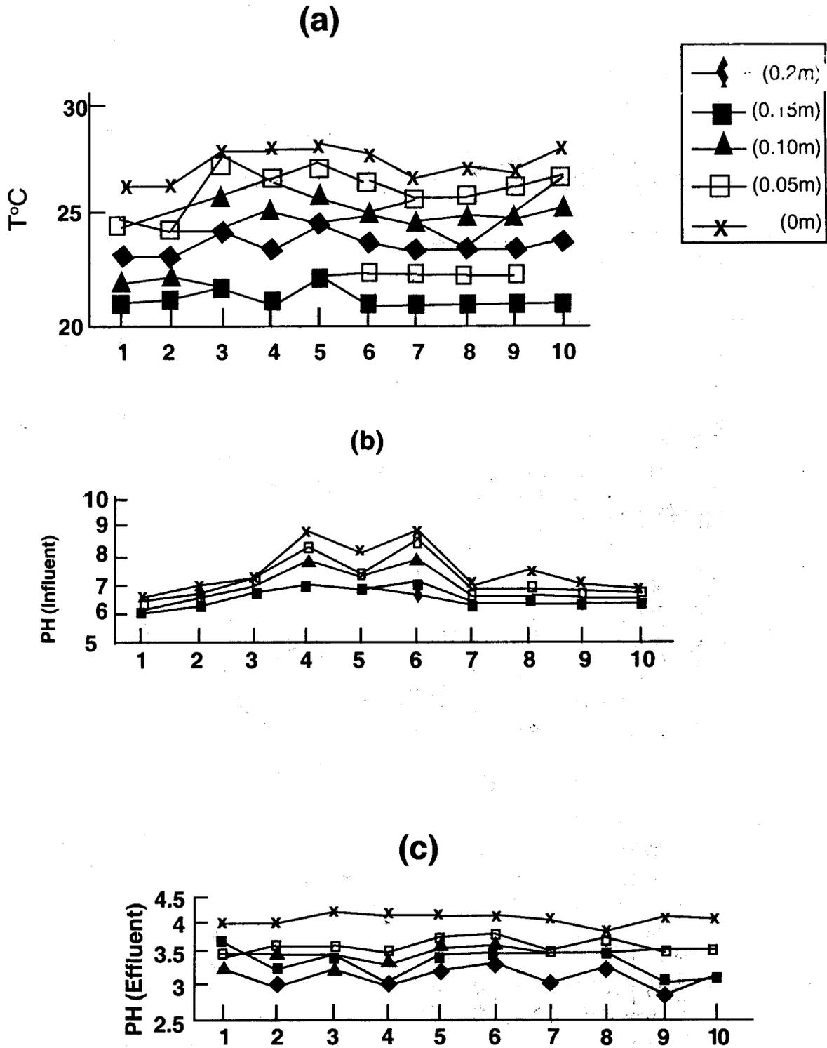
Fig. 2: Weekly Variation of Temperature and PH in WSP at various depths.
