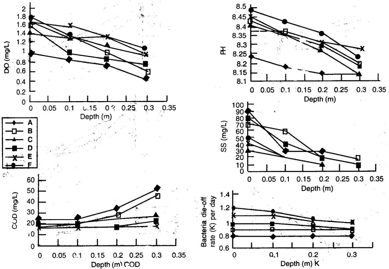
Fig. 6: Variation of DO, PH, T, SS, COD and K with depth due to temperature differences (Day 2).
