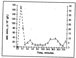
Fig. 3a: Sediment concentration with time.
