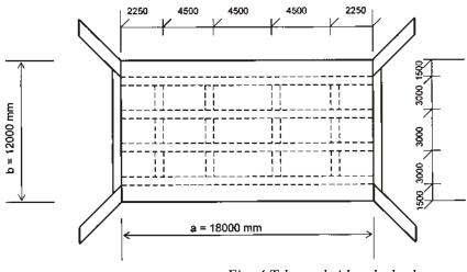
Fig. 4 T-beam bridge deck-plan
