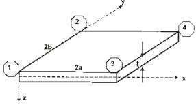
Fig. 2 Co-ordinate system for the plate element
