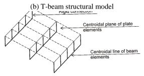
Fig. 1 Beam-plate structure idealisations
