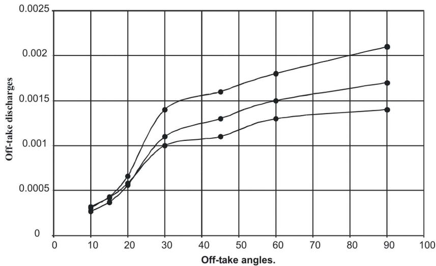
Fig.6: Plot of measured and predicted off-takes against off-take angles for Q19.
