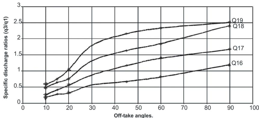
Fig. 2: Effect of off-take angles on specific discharge ratios for flows at concave channel bifurcation
