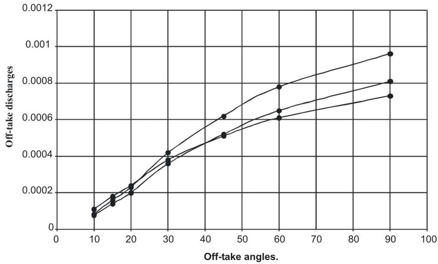
Fig.4: Plot of measured and predicted off-take discharges against off-take angles for Q17.
