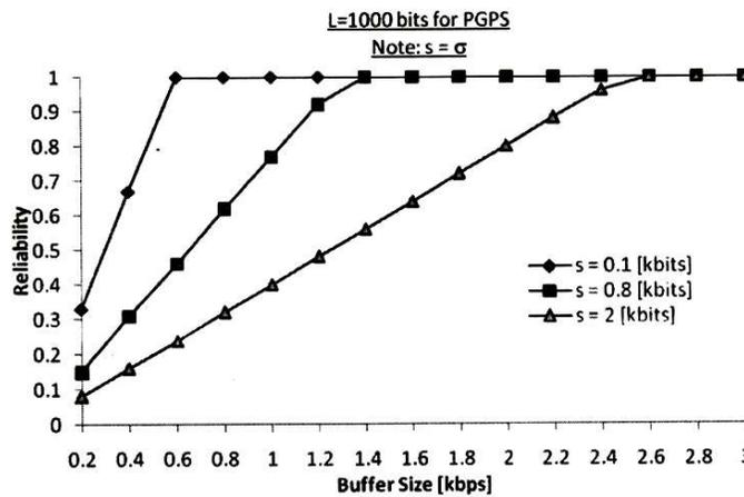
Figure 10: Reliability versus buffer size for only PGPS technique.
