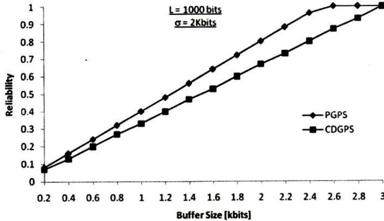
Figure 5: Reliability versus buffer size for both CDGPS and PGPS
