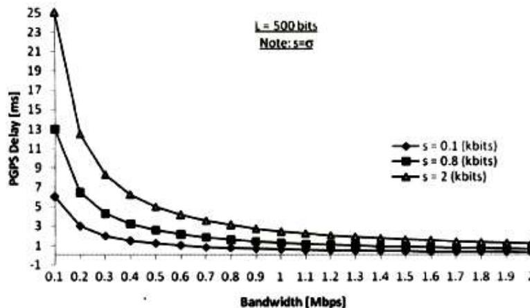
Figure 8: Delay [ms] versus bandwidth [Mbps] for only PGPS technique
