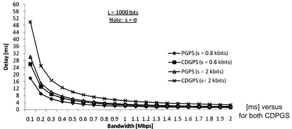
Figure 3: Delay bandwidth [Mbps] and PGPS
