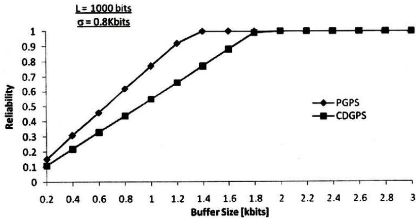
Figure 6: Reliability versus buffer size for both CDGPS and PGPS techniques
