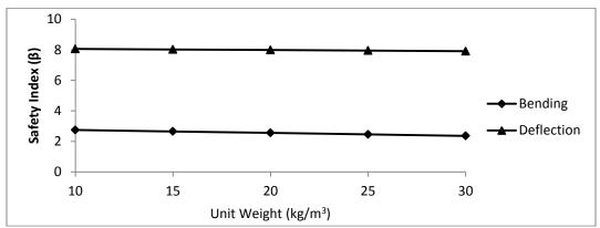
Fig. 6: Safety Index – Unit weight relation for the Nigerian Abura bridge beam
