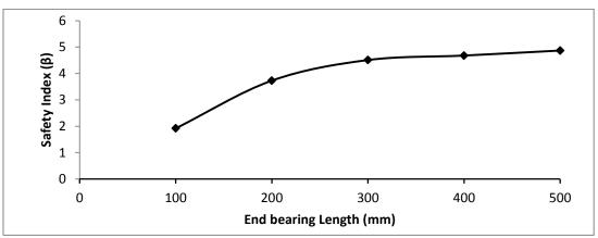
Fig. 8: Safety Index - End bearing length relation for the Nigerian grown Abura bridge beam
