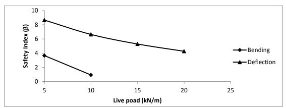
Fig. 4: Safety Index - Live Load relation for the Nigerian Abura timber bridge beam
