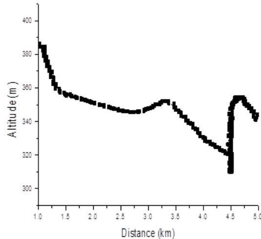
Figure 5: Terrain profile for Pipeline route
