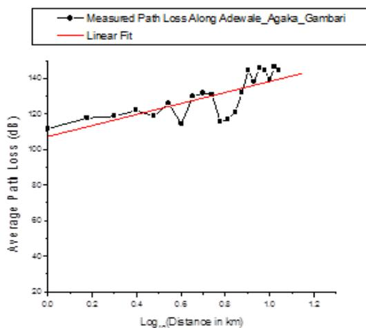
Figure 10: Path loss along Adewale Agaka route
