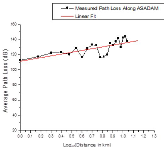
Figure 8: Path loss along ASADAM route
