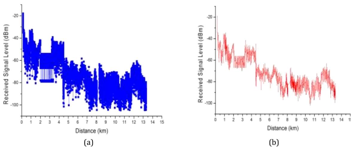
Figure 3: RSL with pick peak, (a) before filtering, (b) after filtering
