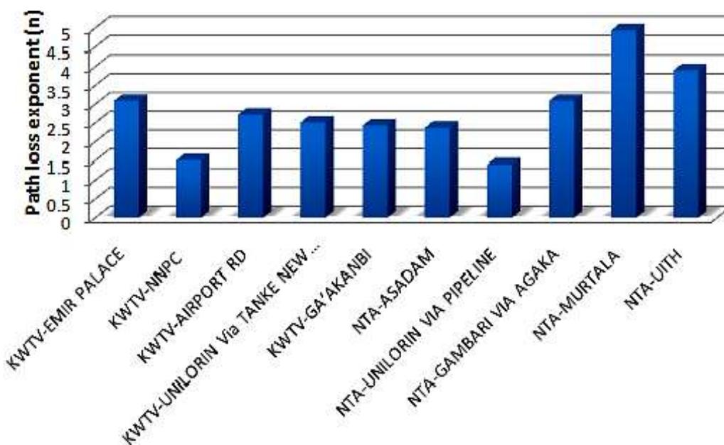
Fig.14: Path loss exponent and measurement routes
