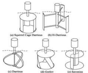
Figure 4: Vertical axis hydrokinetic rotors (Source: [10]).
