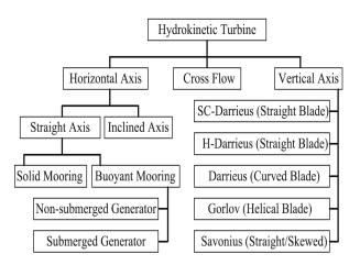
*Figure 2: Classification of hydrokinetic turbines (Source: [8]).*
