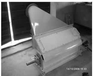
Fig. 13: Crossflow Turbine developed by NASENI Nigerian Journal of Technology
