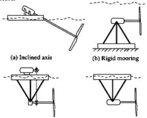
(c) Non-submerged Generator (d) Submerged Generator Figure 3: Axial (horizontal axis) hydrokinetic rotors (Source: [10]).
