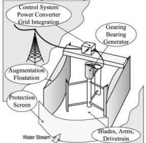
Figure 1: Sketch of a typical Hydrokinetic Turbine System (Source: [8])
