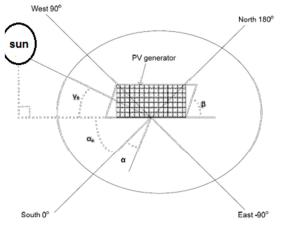
Figure 1: Schematic presentation of the inclination angle of a PV module [8]
