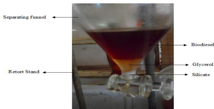
Plate 1: Biodiesel – glycerol - silicate separation
