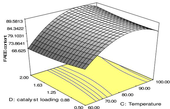
Figure 4: Profile of response surface of biodiesel yield with catalyst loading and Temperature
