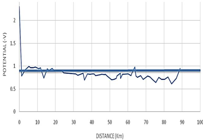
Figure 1: Cathodic Protection Survey on Pipe/Soil Potential test on system 2A pipeline (Warri Pump Station, Benin depot) showing the deviation of the pipe/soil potential values from the standard value, -0.85V.
