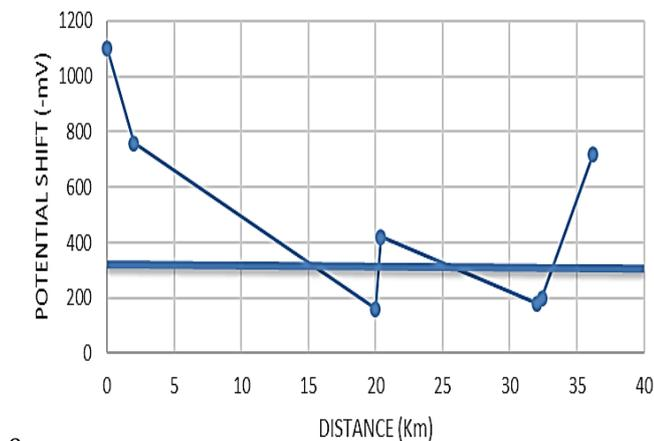
Figure 3: Potential shift on system 2A pipeline (Warr-Amukpe Segment)
