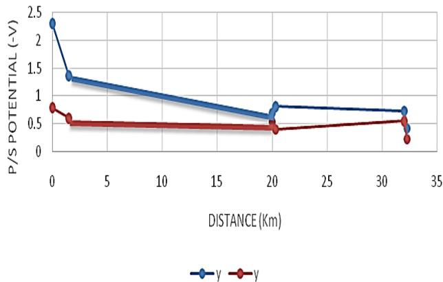
Figure 2: Pipe/Soil potential values of natural and impress current applied status of system 2A pipeline (Warri-Amukpe Axis)
