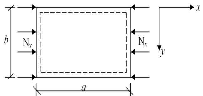
Figure 1: Analytical Model: Rectangular Thin Plate Element with Uniform Compression.
