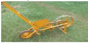
Figure 6: Picture of the completed planter
