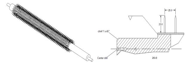
Figure 6 Peeler Shaft for Type 2 Cassava Peeling Machine (Shorter Spikes) 20mm
