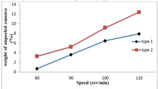
*Figure 10: Graph of Weight of Unpeeled Cassava against the Speed of the Peeling Shaft (Type 1 and 2)*
