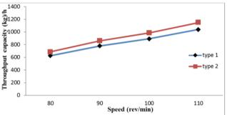
*Figure 14: Graph of Throughput Capacity against the speed of the Peeling Shaft for Machine (Type 1 and 2)*
