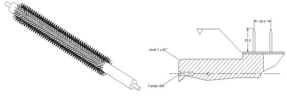
Figure 5 Peeler Shaft for Type 1 Cassava Peeling Machine (Longer spikes) 26mm
