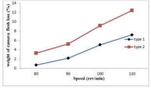
Figure 9: Graph of Weight of Cassava Flesh Loss against the Speed of the Peeling Shaft (Type 1 and 2)
