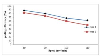
*Figure 12: Graph of Peeling Efficiency against the Speed of the Peeling Shaft (Type 1 and 2)*
