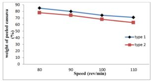
*Figure 7: Graph of Weight of Peeled Cassava against the Speed of the Peeling Shaft (Type 1 and 2)*
