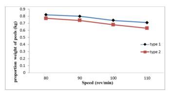
*Figure 11: Graph of Proportion weight of Cassava Peels against the Speed of the Peeling Shaft (Type 1 and 2)*
