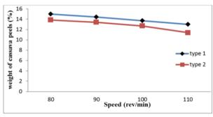
*Figure 8: Graph of Weight of Cassava Peel against the Speed of the Peeling Shaft (Type 1 and 2)*
