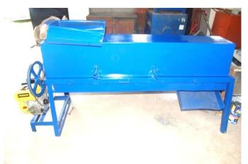
Figure 4 Picture of the Side View of Type 2 Cassava Peeler
