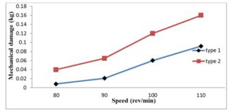
*Figure 13: Graph of Mechanical Damage against the Speed of the Peeling Shaft for Machine (Type 1 and 2)*
