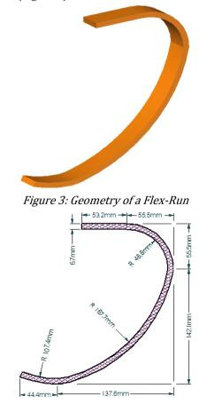
Figure 4: Front View of a Flex-Run
