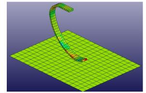
*Figure: 6. LS-DYNA model of a Flexrun impacting on the ground surface*
