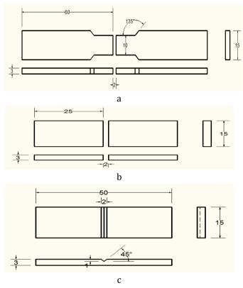
*Figure 2: Standard Joint Preparations samples for tensile, hardness and impact tests in mm.*
