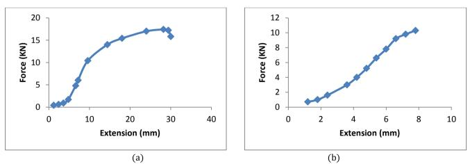
Figure 6: Load-Extension Curve of tensile test on (a) unwelded ASS (C) and (b) welded ASS (C<sub>4</sub>)
