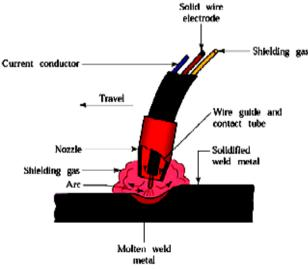
Figure 1: Gas Metal Arc Welding operation [2].
