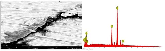
Figure 13: Micrograph of the HAZ of sample C<sub>1</sub> welded and immersed in HCl for 40 days with EDS profile.
