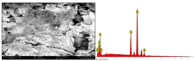
*Figure 12: Micrograph of the control sample immersed in HCl for 40 days with EDS profile*
