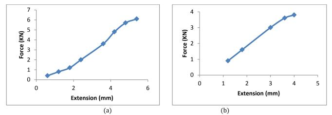
Figure 7: Load-Extension of tensile test on (a) welded ASS ( $C_2$ ) in HCl for 16 days and (b) on welded ASS ( $C_5$ ) in HCl for 40 days
