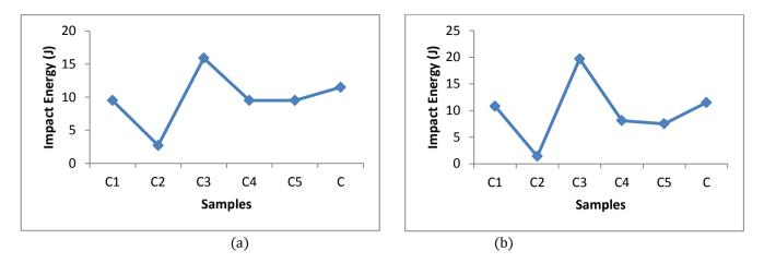
Figure 9: Impact Energy for ASS immersed in HCl for (a) 16 days and (b) 40 days as compared to controls
