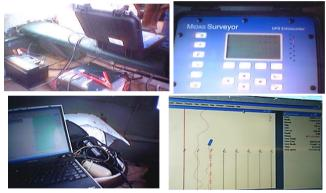
*Figure 3: Survey Boat, MIDAS Surveyor Echo Sounder, Toshiba Laptop and Hypack Navigation System software window.*
