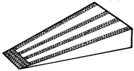
Fig. 8: Stringer bead hardfacing pattern for large aggregates [53]
