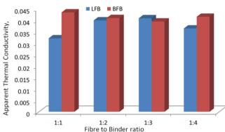
Figure 3: Comparison of Thermal Conductivity of LFB and BFB at different composition
