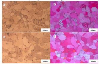
*Fig. 5: Optical micrographs of the solution treated aged samples (a-b) 1 hour, (c-d) 48 hours, images (b, d) are polarized images.*
