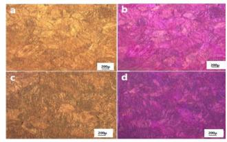
*Fig. 4: Optical micrographs of the non-solution treated* samples aged for (a-b) 1hour (c-d) 48 hours, Images (b, d) are polarized images.
