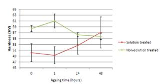
Fig. 2: Comparison of the hardness values of Mg-Zn-Ca alloy samples aged with and without solution heat treatment at 180°C
