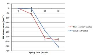
*Fig. 8: Relative TEP measurements of solution treated and non-solution treated samples at different ageing times*
