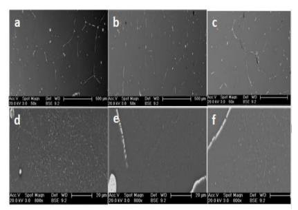
*Fig. 6: SEM micrographs of non-solution treated samples at (a, d) without ageing (b, e) 24hours (c, f) 48 hours ageing times.*
