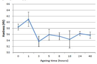
*Fig.1: Age Hardening of Mg-Zn-Ca alloys at 180°C without solution treatment*
