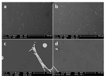
Fig. 7: SEM micrographs of the solution treated samples at ageing times (a-b) 1hour (c-d) 48 hours.
