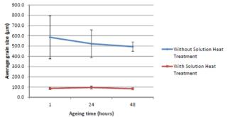
*Fig. 3: Average grain size measurements for aged Mg-Zn-Ca samples with and without solution heat treat treatment*
