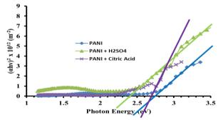
Figure: 2. Plot of (αhv)<sup>2</sup>versus Photon Energy (eV) for pure PANI, PANI + H<sub>2</sub>SO<sub>4</sub> and PANI + Citric acid
