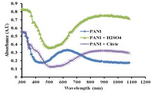
*Figure: 1. Plot of Absorbance against wavelength (nm) for Polyaniline thin films*
