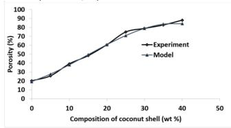
Figure 3: Experimental and model validation showing porosity as a function of the amount of coconut shell particulates
