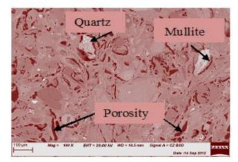
Plate 1: 0% additive fired at at 1150°C, Scale: 100µm
