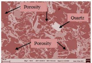
Plate 2: 40 % additive fired at 1150°C, Scale: 100  $\ \mu m$
