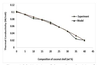
Figure 1 (a): Variation of thermal conductivity of Osiele bricks with % composition of coconut shell particulate, experimental and model
