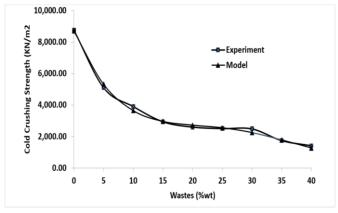
Figure 6: Experiment and model Validation showing CCS as a function of percentage composition of coconut shell particulates.
