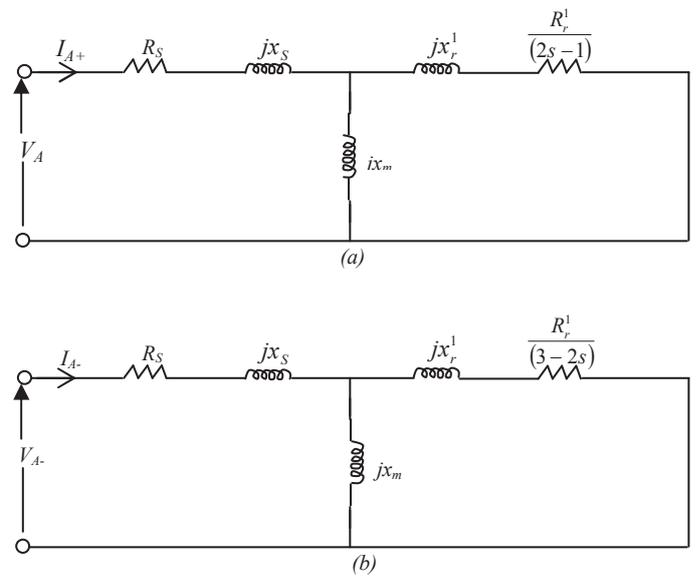
Figure 5: Per phase-sequence networks of the 3-phase TF machine (a) Positive (b) Negative.
