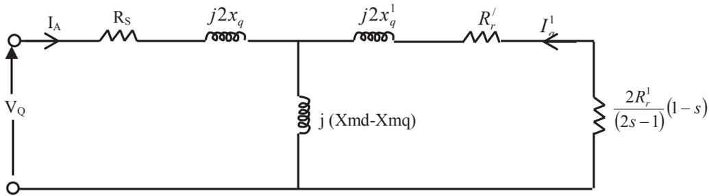
Figure 3: Per-phase steady-state equivalent circuit of polyphase TF machine operating in the asynchronous mode.
