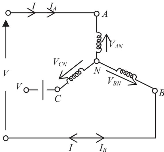
Figure 4: Single-phase operation of a 3-phase TF machine with line C disconnected.
