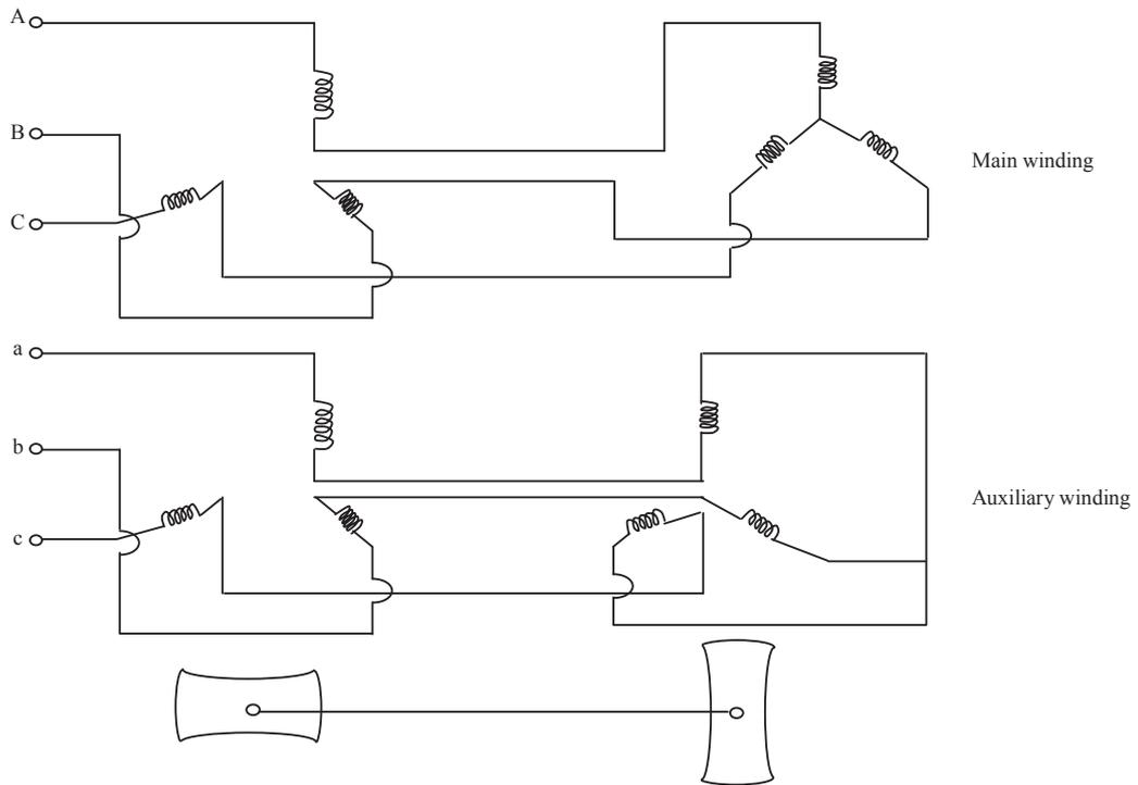
Figure 1: Physical configuration of the polyphase TF machine.
