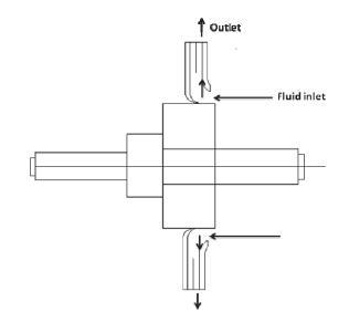
Figure 5: Radial flow impeller.
