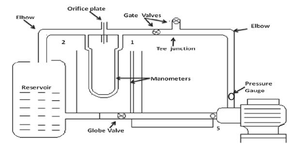
Figure 1: Simplified diagram of the demonstration unit.
