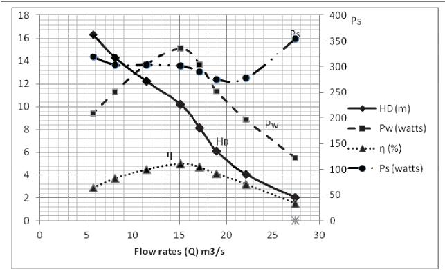
Figure 6: Pump performance characteristics.
