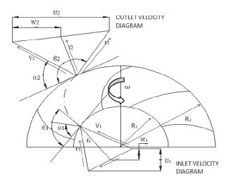
Figure 4: Velocity diagram for pump impeller.
