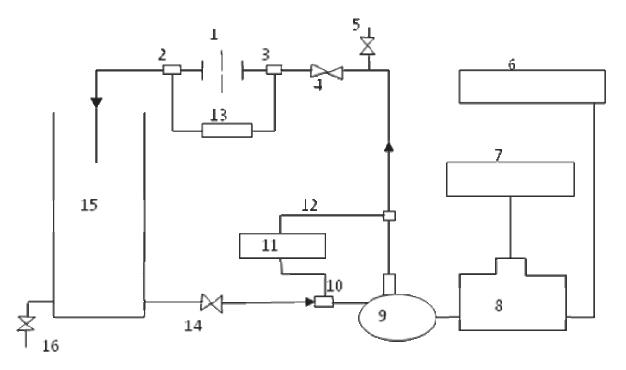
Figure 2: Line diagram of the demonstration unit. (1) Orifice Plate, (2) Low pressure area, (3)High Pressure area, (4) and (5) Gate Valves, (6) Motor Speed (rpm), (7) Motor power (watts), (8) Motor, (9) Pump, (10) Low pressure area (Pump suction), (11) Differential Pressure across pump (KPa), (12)High pressure area (Pump delivery)(13) Differential Pressure across Orifice (KPa), (14) Globe Valve, (15) Reservoir, (16) Drain.
