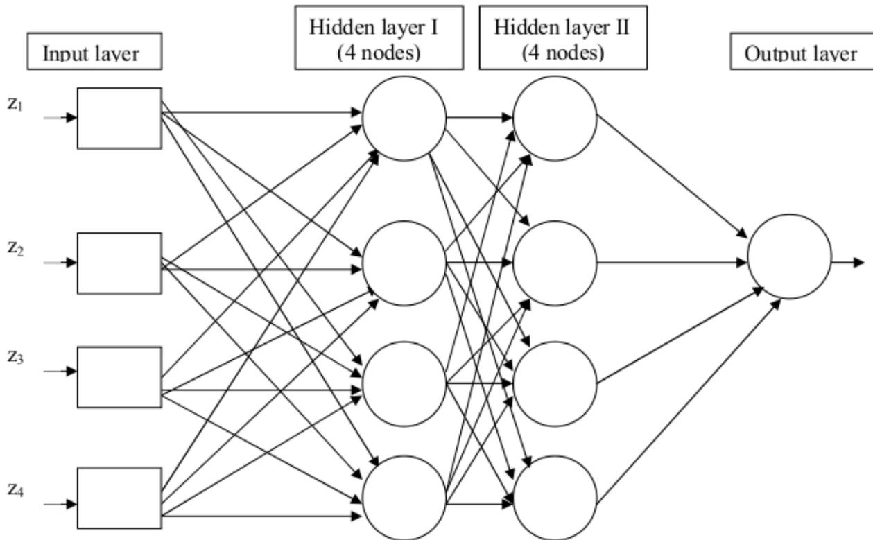
Figure 3: The Four-input, 4 layers feed forward neural network model.
