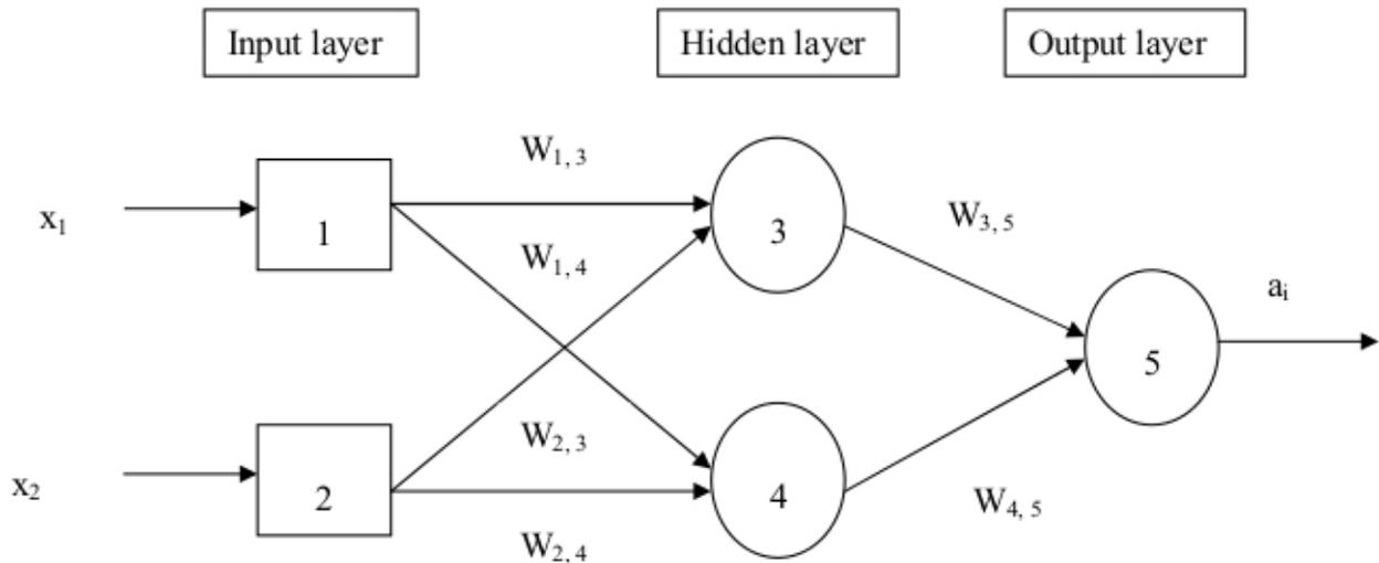
Figure 2: Two-input feed forward neural network model.
