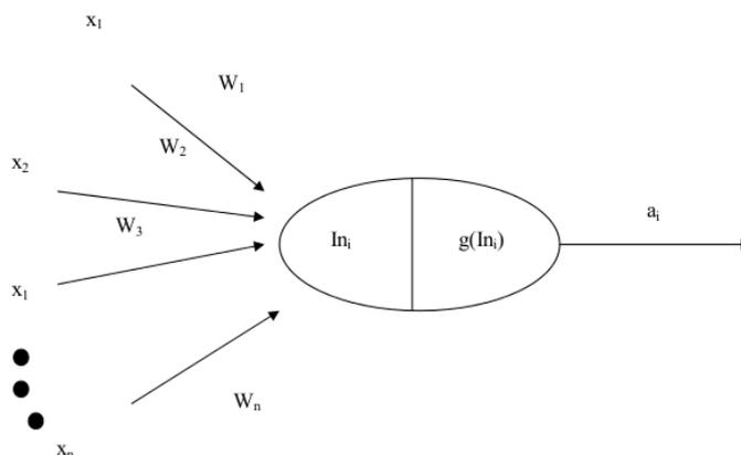
Figure 1: An artificial neuron. ( $W_i$  = weights;  $x_i$  = inputs;  $a_i$  = output)
