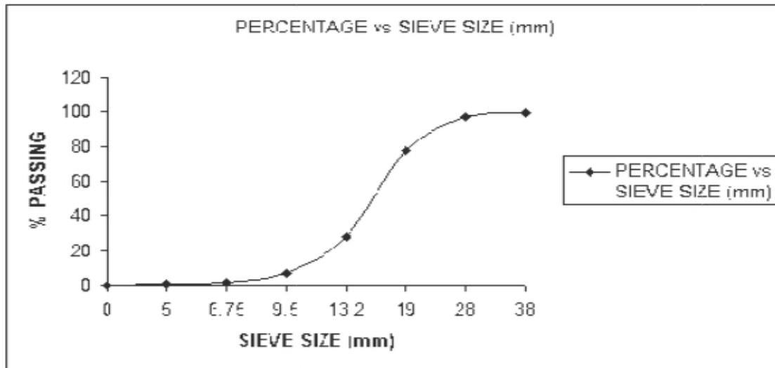
Figure 5: Grading curve for granite.
