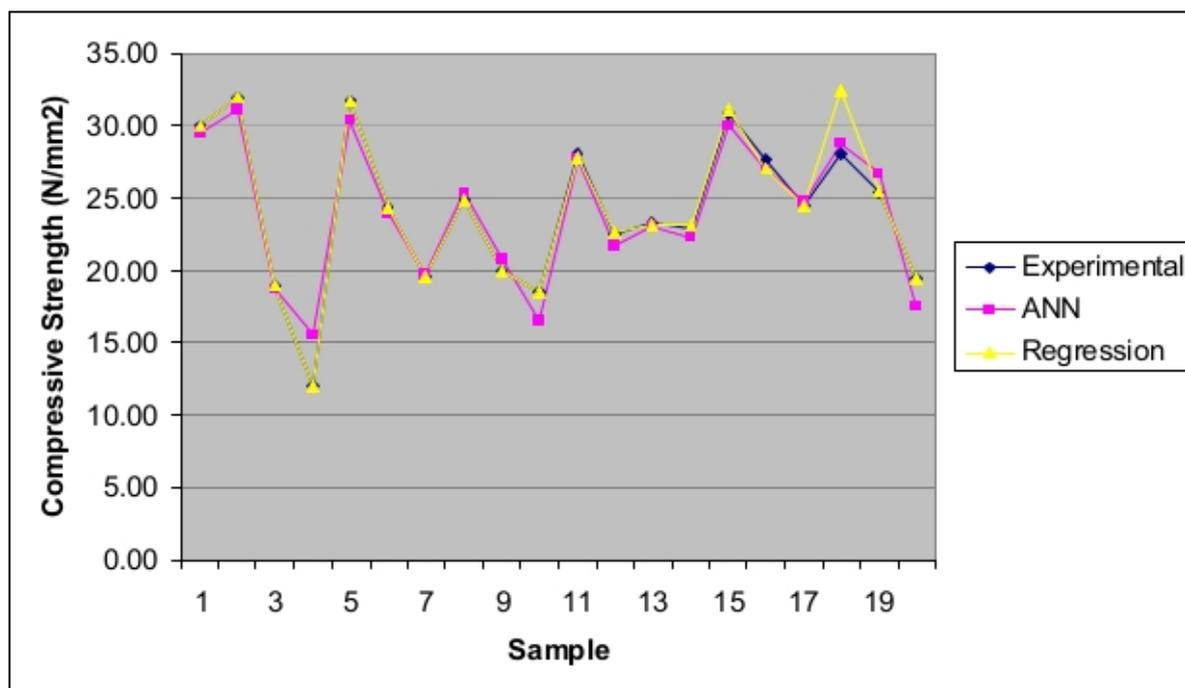
Figure 6: Comparison of ANN with experimental results and regression model prediction (granite).
