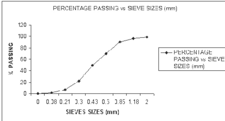
Figure 4: Grading curve for the fine aggregate.
