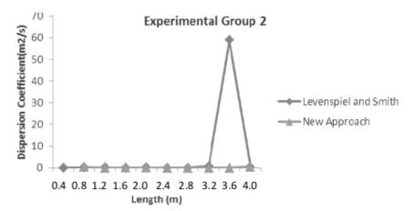
Figure 4: Variation of Dispersion Coefficient with Sampling Length for Experiment 2.
