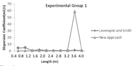
Figure 2: Variation of Dispersion Coefficient with Sampling Length for Experiment 1.
