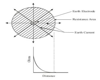
Figure 2: Earth electrode resistance area.
