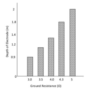
Figure 4: Histogram of test Result from fluke 1625 tester.
