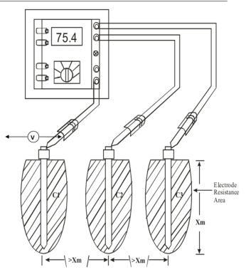
(a) Setup for testing soil resistivity using the fluke 1625
