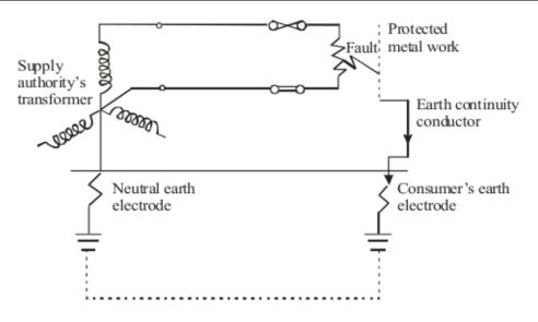
Figure 1: Earth fault loop-path.
