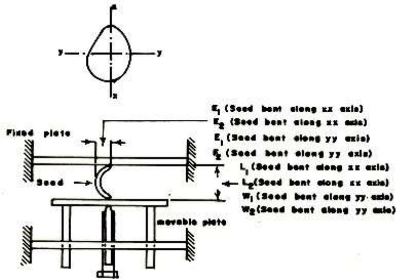
Fig.3. Schematic diagram of the rig built for bending the seeds.
