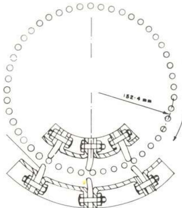
Fig.7. Section at the shelling unit showing the concave in two parts (cylinder rotates in the direction of the arrow).
