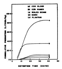
Fig. 2. Cummulative biogas yield from the various waste food materials.
