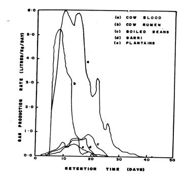
Fig. 3. Biogas production rate from the var10US waste food materials.
