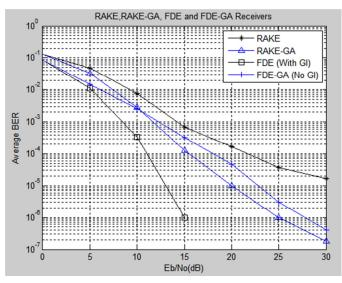
Figure 5: BER vs. Eb/No for all the receivers for CM1.
