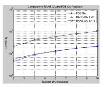
Figure 2: Complexity of RAKE-GA receiver and FDE-GA receiver for CM3.
