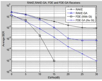
Figure 6: BER vs. Eb/No for all the receivers with similar complexity values for CM3.
