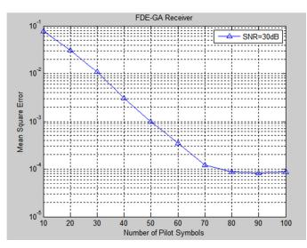
Figure 8: MSE vs. Pilot Symbols for FDE-GA receiver for CM3.
