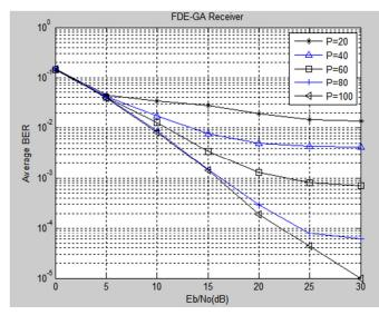
Figure 7: BER vs. Eb/No for FDE-GA receiver for CM3.
