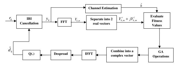
Figure 1: Block diagram of FDE-GA receiver for DS-UWB Systems.
