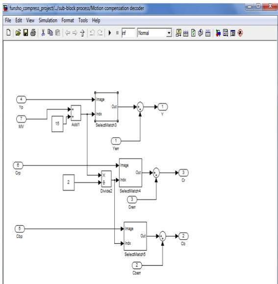
Figure 4: Motion Compensation/Estimation Block.
