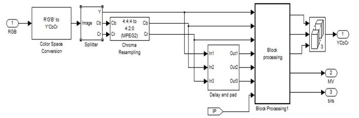
Figure 2: Block Process for the Video Compression (Encoder Block)
