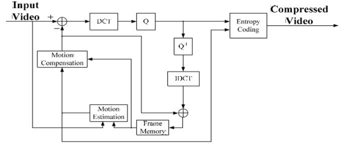
Figure 1: Generalized encoder structure of MPEG
