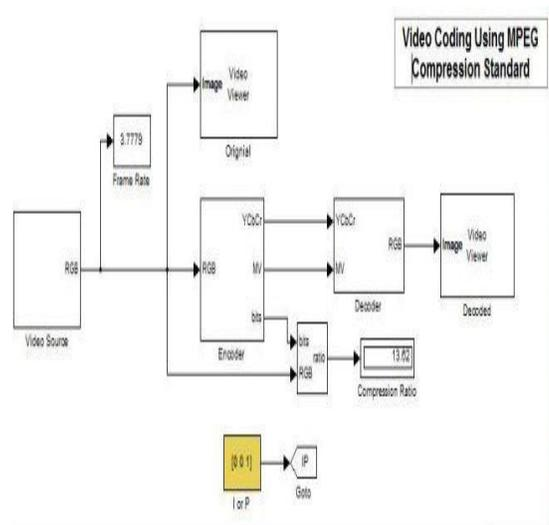
Figure 5: Final Simulink Model for the Video Compression
