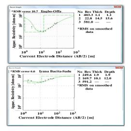
Figure 4b: Typical Schlumberger sounding curves obtained in the study area
