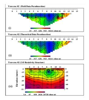
Figure 5b: (i) Field data pseudosection (ii) Theoretical data pseudosection and (iii) 2-D resistivity structure along traverse  $02\,$
