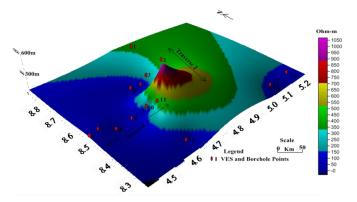
Figure 7: Apparent resistivity 3-D surface for AB/2 equals 50m within the study area
