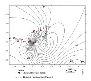
Figure 6: Apparent resistivity contour map for AB/2 equals 50m within the study area
