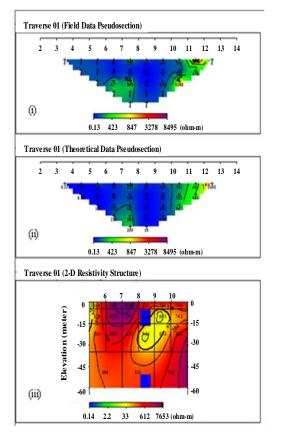
Figure 5a: (i) Field data pseudosection (ii) Theoretical data pseudosection and (iii) 2-D resistivity structure along traverse 01
