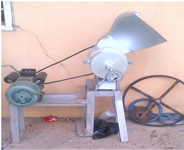
Figure 6: The fabricated cracking machine.
