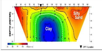
Figure 4a: Inverted resistivity sections along traverse 1
