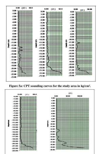
Figure 5b: CPT sounding curves for the study area in kg/cm<sup>2</sup> (contd.).
