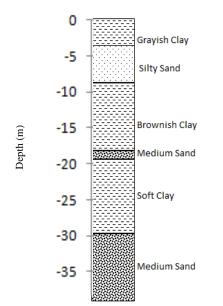
Figure 3: Borehole log showing the sequence of clay and sand in the study area
