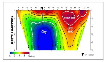
Figure 4d: Inverted resistivity sections along traverse 4
