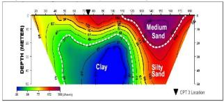
Figure 4c: Inverted resistivity sections along traverse
