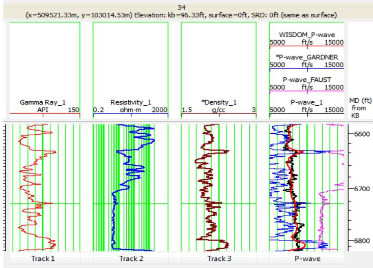
Figure 7: Display of the three different techniques
